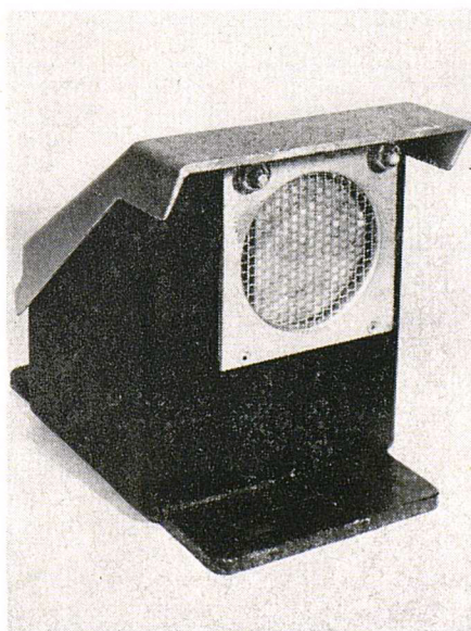
A cast iron case houses the radiometer head at trackside.
